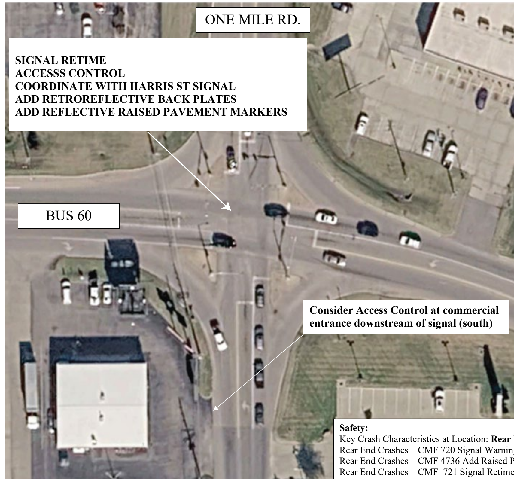
Figure 31: Improvement Option BUS 60 / One Mile Road Intersection
